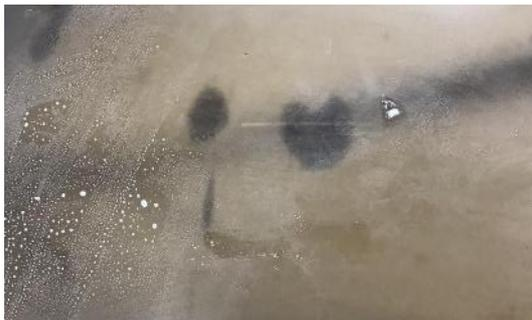
(6) Large surface roughness on surface of parts/residual debris in the tank: 1st, reduce the normal exposure parameters by 20~30% or the other appropriate amount. 2nd, filter the resin in the liquid tank before reprint.
