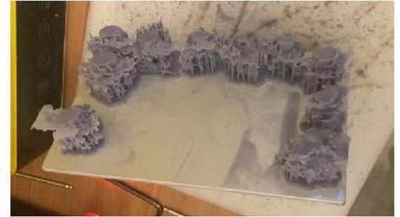
(2) The formed part and the support are disconnected from the support connection: In the slicing software, increasing the depth of the support embedded in the part (0.5mm), increase the support diameter, and the support distance/density appropriately .
