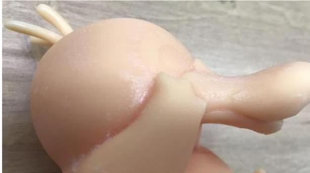
(9) The whole surface exposure layer appears in the printing process: a. Check the slice image of the whole layer in the slice data, and check whether there is any error in the original stl file; b. The LCD printer screen abnormally exposes /DLP light machine exposes: restart the device / contact the after-sales service.
